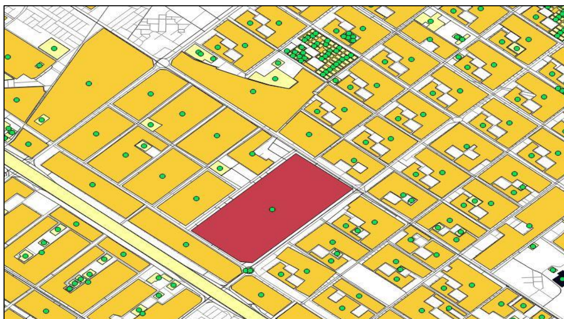
Figure 4. A sample of output for the process of specifying the center of polygons.
