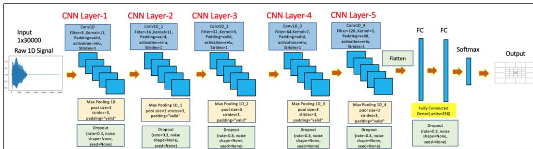
Figure 2. 1D CNN configuration with parameter adjustment
