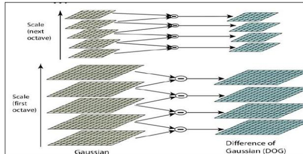
**Figure 5. Construction of difference-of-Gaussian images**
