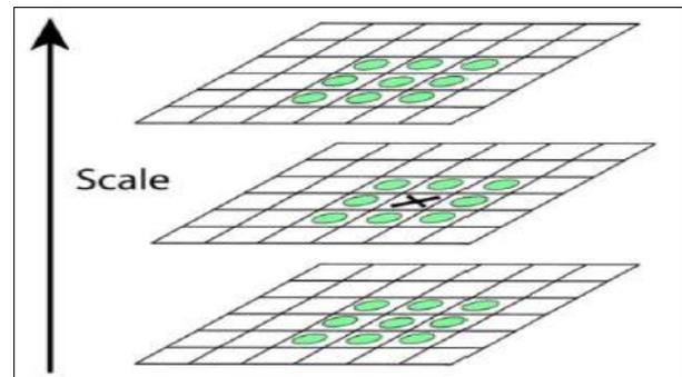
**Figure 6. “Pixel assessments to find the difference-of-Gaussian image's maximum and minimum values”**
