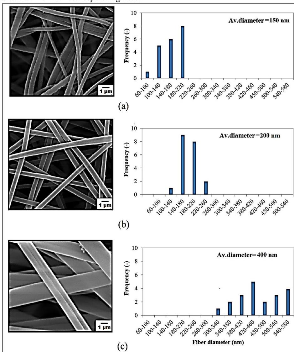
**Figure 2. SEM images of PAN-based EPNF membranes (magnification is 10000 X) and the corresponded fiber size prepared from different PAN/DMF concentrations (a) 8%PAN/DMF, (b) 11%PAN/DMF, and (c) 14%PAN/DMF.**
