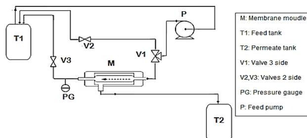
**Figure 1. Schematic diagram of the cross-flow filtration system**
