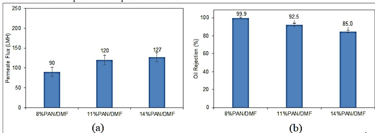
**Figure 3. The separation efficiency of the different fabricated EPNF membranes used in oil filtration at baseline conditions (Feed flowrate= 60 ml/min, feed oil concentration = 250 mg/L, transmembrane pressure = 1.5 psi, and temperature= 25°C) (a) Permeate flux and (b) Oil rejection**
