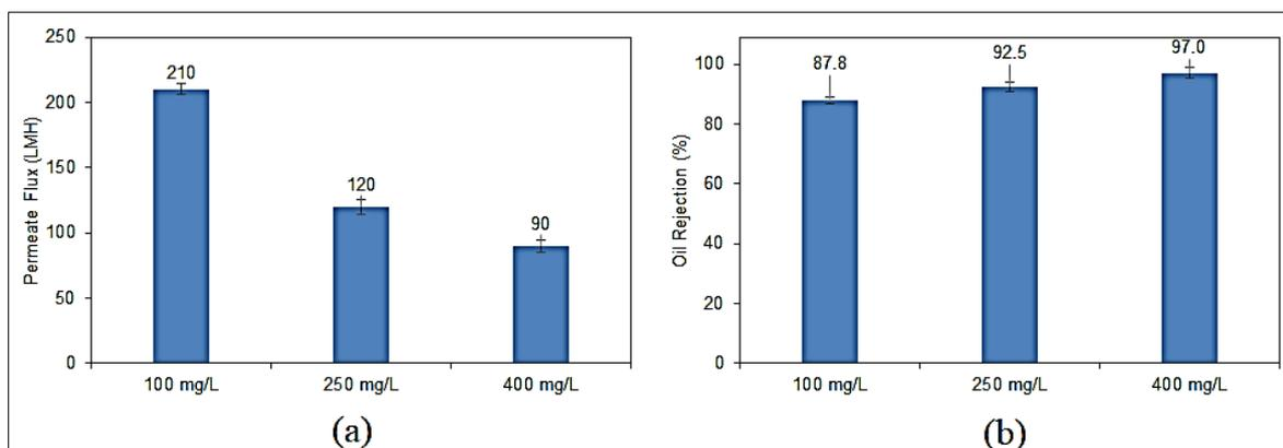
Figure 7. The separation efficiency of 11% PAN/DMF EPNF membrane under various feed oil concentrations (Feed flowrate= 60 ml/min, transmembrane pressure = 1.5 psi, and temperature= 25°C) (a) Permeate flux and (b) Oil rejection
