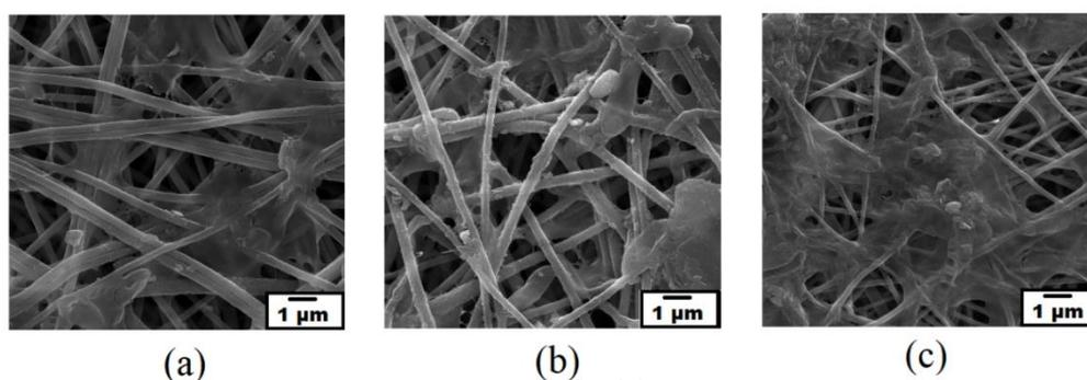
Figure 8. The SEM images of the 11% PAN/DM EPNF membranes (magnification is 10000 X) after emulsified oil removal under various feed oil concentrations (a) 100 mg/L, (b) 250 mg/L, and (c) 400 mg/L.
