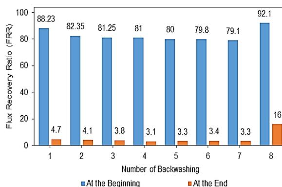
**Figure 11.** The backwashing cycles of 11 wt.% PAN/DMF membrane (Feed flowrate= 60 ml/min, feed oil concentration = 250 mg/L, transmembrane pressure = 1.5 psi, and temperature= 25°C)
