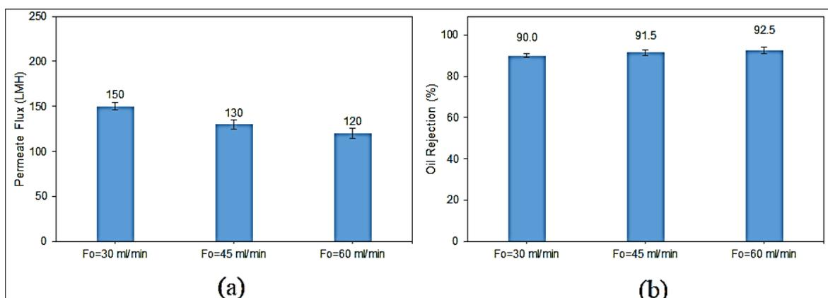
Figure 5. The separation efficiency of 11% PAN/DMF membrane under various initial feed flow rates (feed oil concentration = 250 mg/L, transmembrane pressure = 1.5 psi, and temperature= 25°C) (a) Permeate flux and (b) Oil rejection
