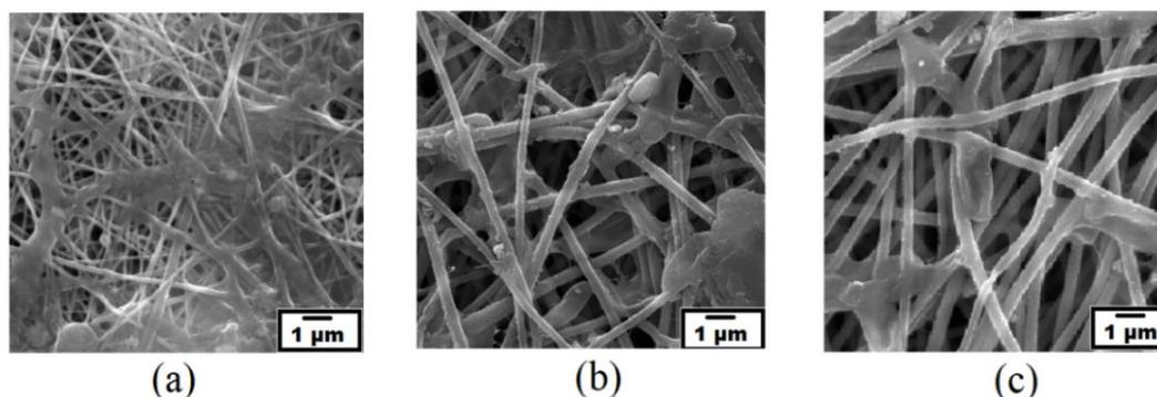
**Figure 4. The SEM images of the different fabricated EPNF membranes (magnification is 10000 X) used in oil filtration at baseline conditions (a) 8% PAN/DMF, (b) 11 % PAN/DMF, and (c) 14 % PAN/DMF**
