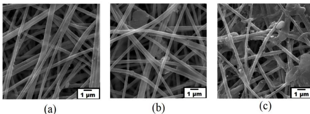
Figure 6. The SEM images of the 11 % PAN/DMF EPNF membranes (magnification is 10000 X) after emulsified oil removal under various initial feed flow rates (a) 30 ml/min, (b) 45 ml/min, and (c) 60 ml/min.
