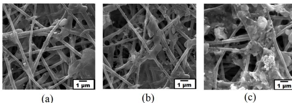
**Figure 10.** The SEM images of the 11% PAN/DMF EPNF membranes (magnification is 10000 X) after emulsified oil removal under various transmembrane pressures (a) 1.5 psi, (b) 5 psi, and (c) 10 psi.
