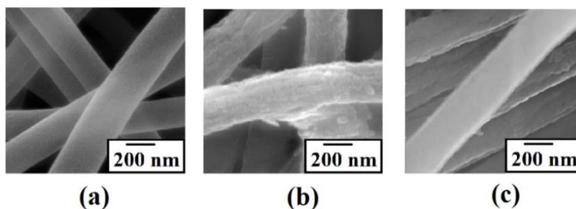
**Figure 12.** High resolution SEM images of the surface of 11 wt. % PAN/DMF membrane (magnification is 160000 X) (a) Clean membrane (b) Fouled membrane, and (c) Backwashed membrane
