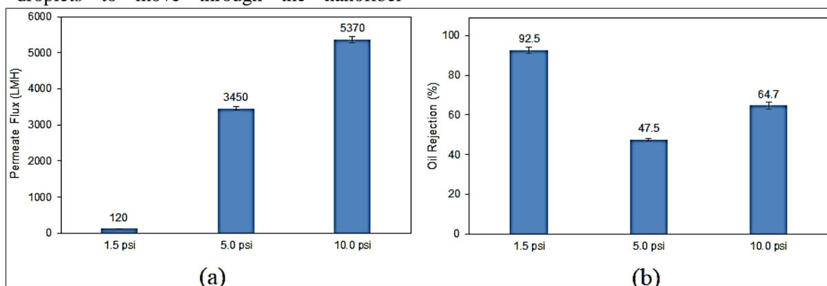
Figure 9. The separation efficiency of 11% PAN/DMF membrane under various transmembrane pressures (Feed flowrate= 60 ml/min, feed oil concentration = 250 mg/L, and temperature= 25°C) (a) Permeate flux and (b) Oil rejection
