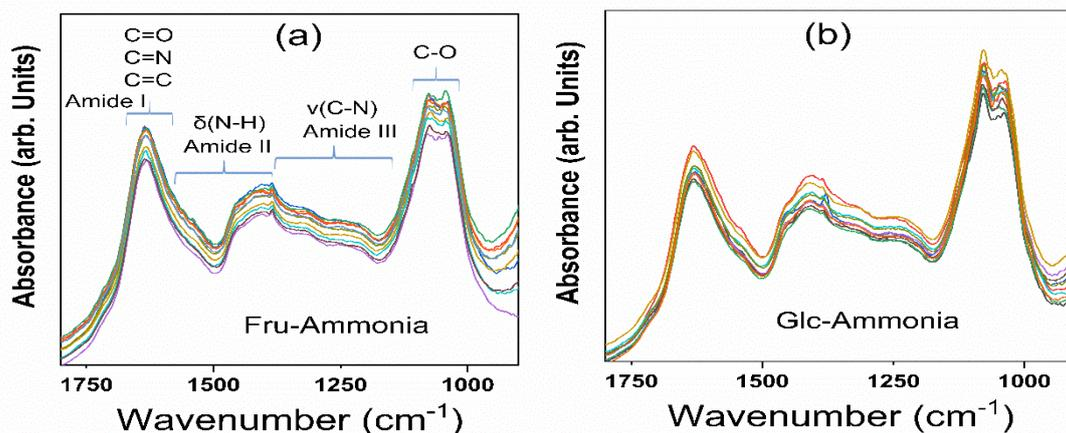
Figure 5. FTIR spectra of melanoidin samples derived from Fru-ammonia (a), and Glc-ammonia (b) in the 1800–900  $\text{cm}^{-1}$  range.
