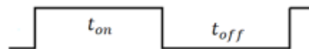
Figure 2. A schematic drawing of glow and afterglow times of a square DC voltage.
