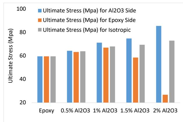
Figure 7. The ultimate stress for neat epoxy and FGMs at difference volume fraction and constant speed ( $N=1200$  r.p. m) and time ( $T=6$  min) for both sides; nano alumina and epoxy
