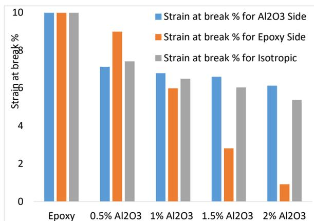
**Figure 8. The strain at break for neat epoxy and FGMs at difference volume fraction and constant speed  $N=1200$  r.p.m and constant time  $T=6$  min for both sides; nano alumina and epoxy.**
