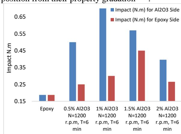
**Figure 10. Impact strength of FGMs alumina particles at different volume fractions and constant speed  $N=1200$  r.p.m and constant time  $T=6$ min**
