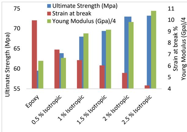
Figure 5. Effect of alumina nano particles on Young's modulus, ultimate strength and strain at break.
