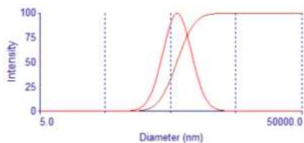
Figure 2. Particle size of  $Al_2O_3$  nanoparticles
