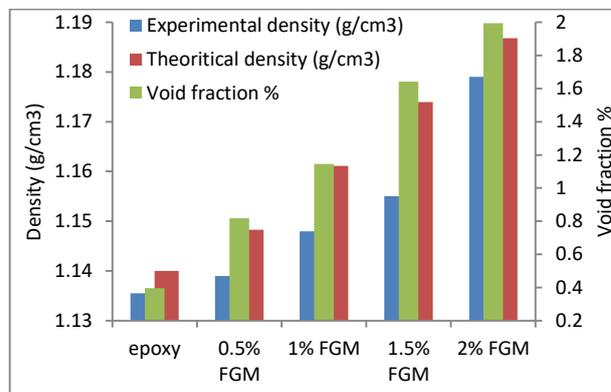
**Figure 4. The theoretical, experimental densities and corresponding void content of the neat epoxy, FGM's (Al<sub>2</sub>O<sub>3</sub>) and equivalent alumina composite**
