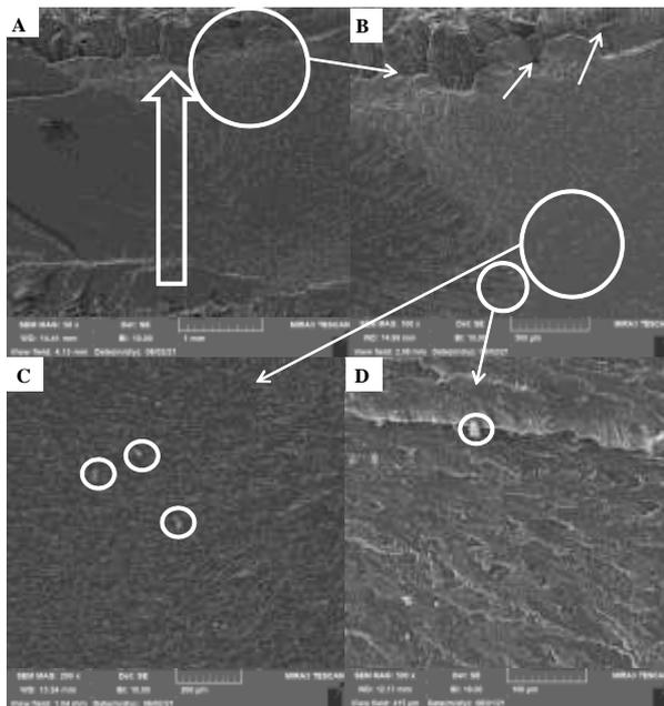
**Figure 12.** SEM images of impact fracture surface of FGM of 2%  $V_f$  of nano-  $Al_2O_3$  with rotational speed  $N=1200$  r.p.m and time  $T= 6$  min with different magnification.
