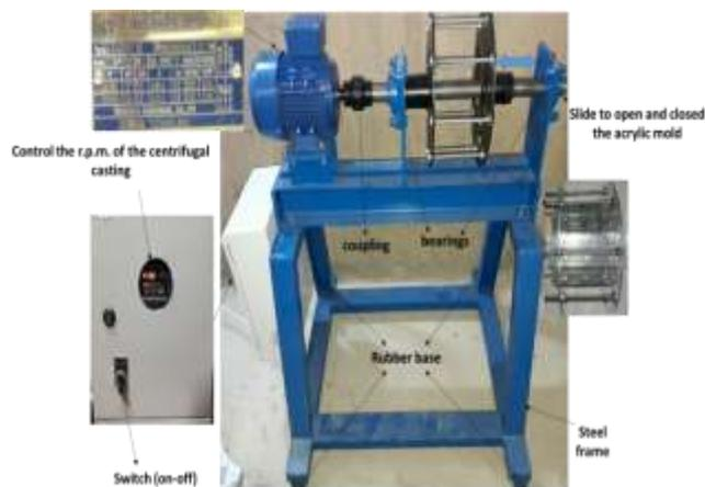
Figure 1. Centrifugal casting apparatus used in this work.
