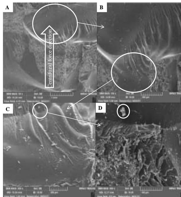
**Figure 11. SEM images of the impact fracture surface of FGM of 0.5% nano  $Al_2O_3$  with rotational speed  $N=1200$  r.p.m and time  $T= 6$  min with different magnification.**
