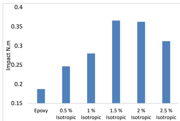
**Figure 9. Shows impact strength of neat epoxy and homogenous composite material.**
