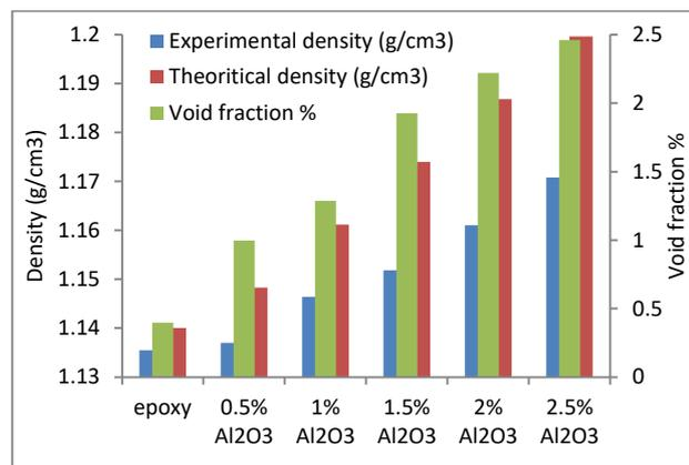
**Figure 3. The theoretical, experimental densities and the corresponding content of void of the neat epoxy and alumina nano-composite at different volume fraction.**
