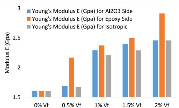
Figure 6. The Young's Modulus for neat epoxy and (FGMs) at difference volume fraction and constant speed ( $N=1200$  r.p.m) and time ( $T=6$  min) for both sides; nano alumina side and epoxy side
