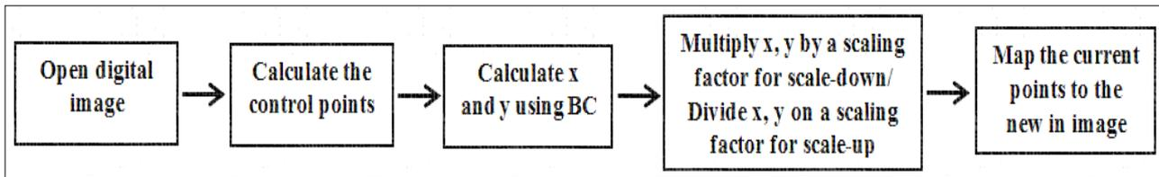
Figure 2. Block diagram for scaling-up and scaling-down.
