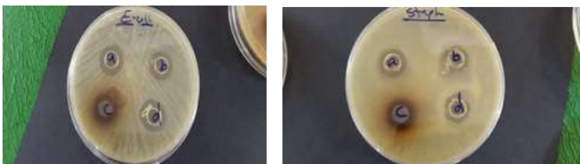
Figure 4. Antibacterial test against *Escherichia coli* and *Staphylococcus aureus*, for nanocomposite P<sub>2</sub> with different weight of Ag, a= P<sub>2</sub>/Ag 1%, b= P<sub>2</sub>/Ag 3%, c= P<sub>2</sub>/Ag 5%, d= P<sub>2</sub>/Ag 7%.
