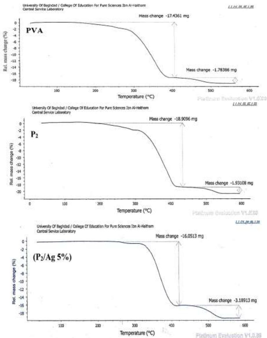
Figure 5. The TGA of PVA, P<sub>2</sub> and nanocomposite (P<sub>2</sub>/Ag 5%)
