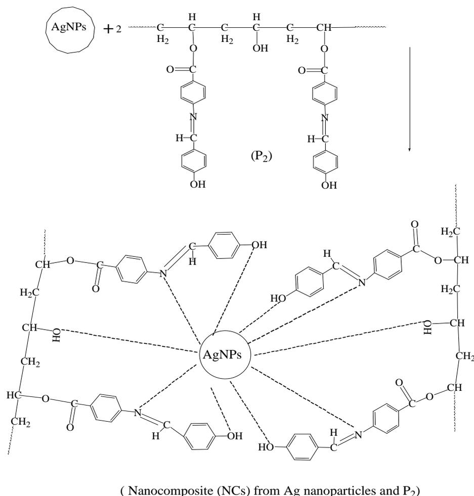
Figure 2. Process of synthesizing nanocomposite (NCs) from Ag nanoparticles and P<sub>2</sub>
