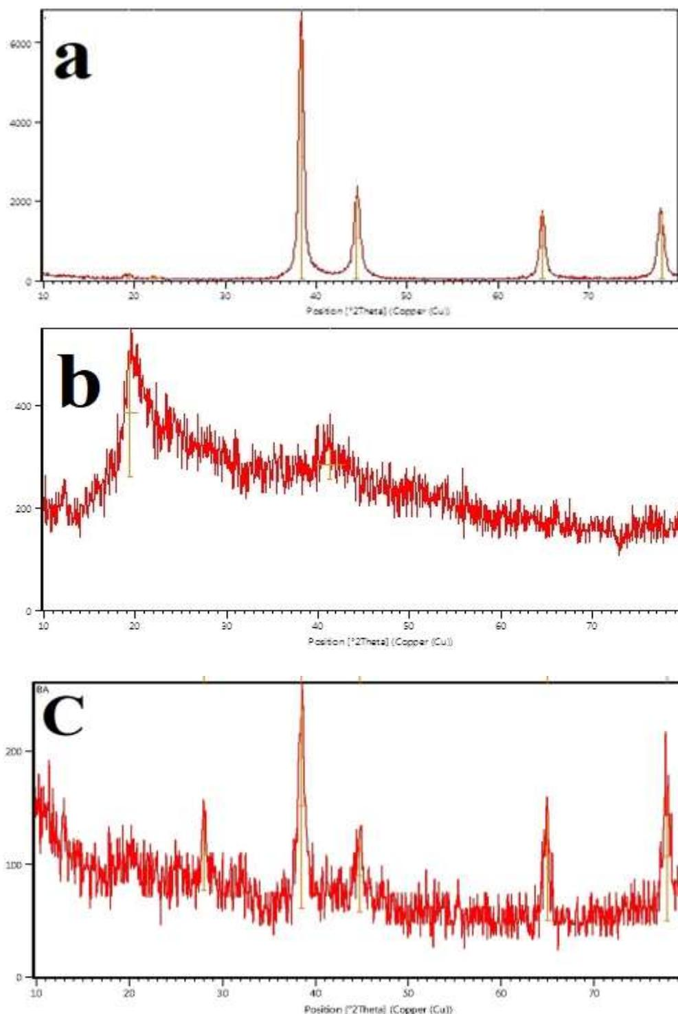
Figure 6. XRD of PVA=a, P<sub>2</sub> =b and nanocomposite (P<sub>2</sub>/Ag 5%) = c
