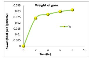
Figure 3. Weight gain from single-stage coating (alluminization only) at 1000 °C as a function of time for AISI304
