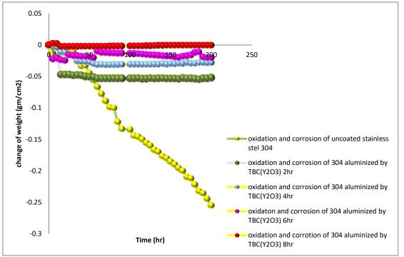
Figure 9. Oxidation and hot corrosion of the coating with the presence of the thermal barrier Y<sub>2</sub>O<sub>3</sub> for the alloy for the time periods 2, 4, 6, 8 hours.
