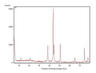
Figure 6. X-ray diffraction plot of a sample coated with aluminum at 1000 °C for 8 hours
