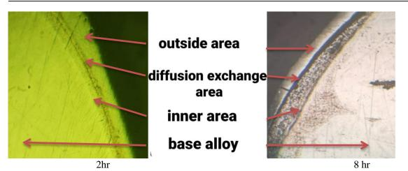
Figure 5. Microstructure of the samples coated with a single-phase (alluminization only) at a temperature 1000 °C for 2 and 8 hour periods
