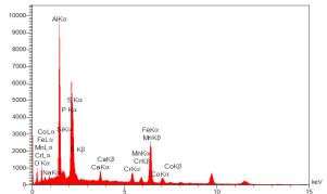
Figure 8. Scheme of quantitative and qualitative examination by scanning electronic device (SEM-EDS) for austenitic stainless steel alloy (AISI-304) coated with single aluminum for 6hr at a temperature of 1000 °C.
