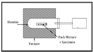
Figure 1. A schematic diagram showing the coating process in an electric furnace.
