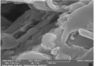
Figure 7. Microscopic structure by scanning electron device (SEM) of austenitic stainless steel (AISI-304) alloy coated with single aluminum for 6hr at 1000 °C.
