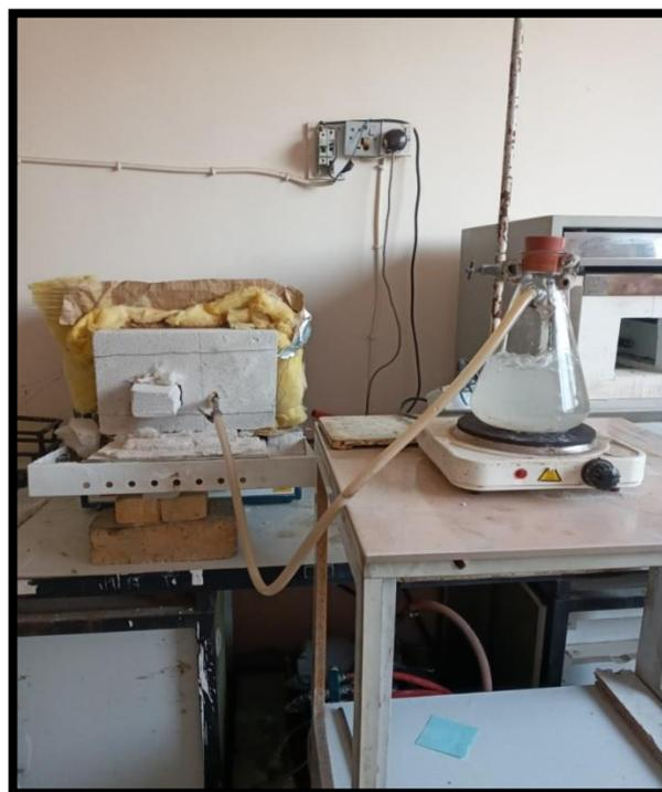
**Figure 2.** The system used in the cyclic oxidation process
