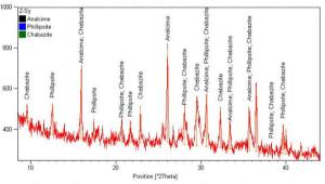
Figure 4. XRD spectrum of studied zeolite
