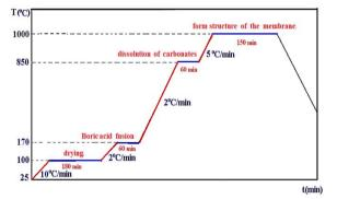
Figure 3. program of thermal treatment of prepared ceramic membrane
