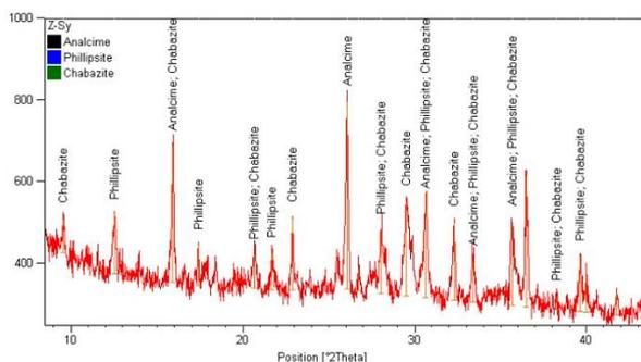
Figure 4. XRD spectrum of studied zeolite
