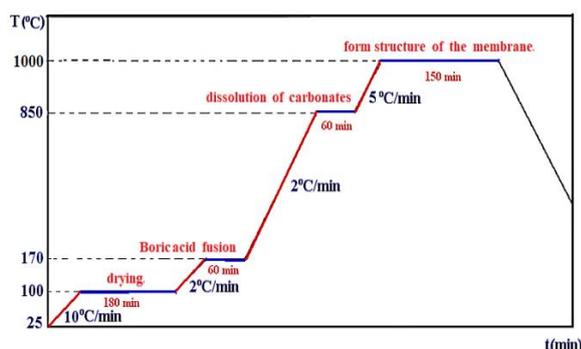
Figure 3. program of thermal treatment of prepared ceramic membrane
