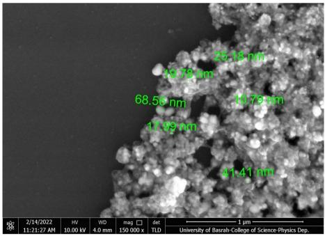
Figure 8. SEM micrograph of the synthesized qrdAgNPs by aqueous extract of *T. domingensis* pollen grains (qurrait).
