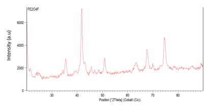
Figure 4. Diffraction spectrum of iron oxide
