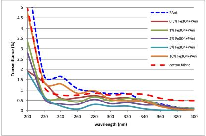
**Figure 6. UV transmittance spectra of treated cotton fabrics**
