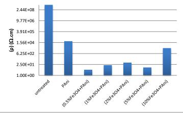
Figure 5. specific electrical resistivity of cotton samples
