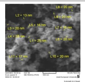
Figure 3. Micrograph of a (Fe<sub>3</sub>O<sub>4</sub>) powder
