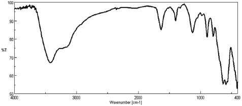
Figure 1. Infrared spectrum of iron oxide prepared using iron (II and III) sulfate
