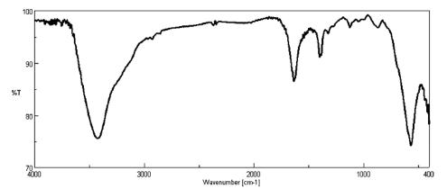
Figure 2. Infrared spectrum of iron oxide prepared using iron (II and III) chloride
