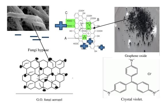
Figure 16. Graphiane oxide fungi aerogel and interaction with crystal violet
