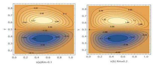
Figure 9. Impact of magnetic Reynolds numbers Rm on the stream lines
