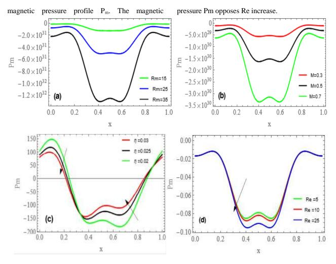
Figure 5. Magnetic pressure profiles for different fluid parameters.
