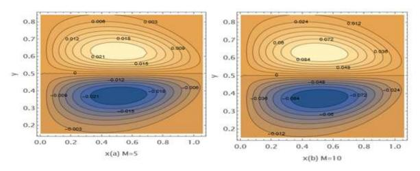
Figure 7. Impact of Hartmann number *M* on the stream lines
