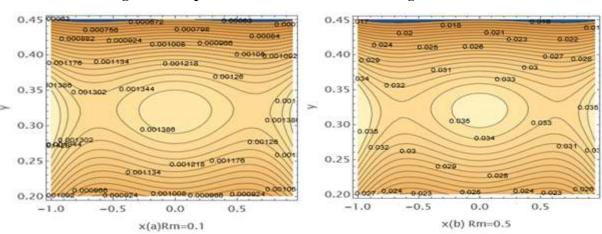
Figure 11. Impact of electrical field E on the magnetic force contours
