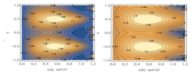
Figure 8. Impact of permeability parameters  $\eta$  on the stream lines
