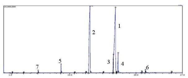
Figure 4. Chromatogram of biodiesel at optimum conditions by using GC-MS
