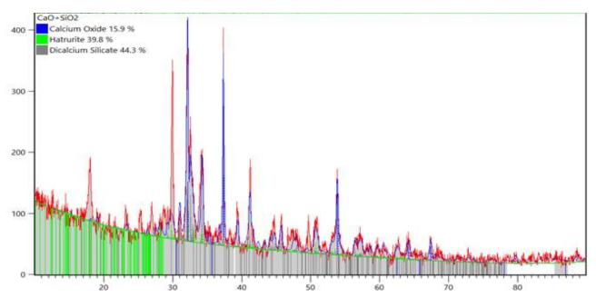
Figure 2. XRD diffraction pattern of CaO impregnated on SiO<sub>2</sub> catalyst
