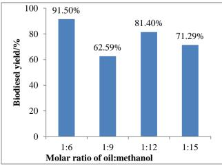
Figure 3. The relationship between the molar ratio of oil to methanol and biodiesel yield in the transesterification of RBDPO with 3% CaO/SiO<sub>2</sub> catalyst
