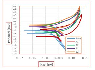
Figure 8. Cycle polarization curves of  $TiO_2$ , and  $ZrO_2/TiO_2$  coated by PEO process and base at different time and applied voltages 400V in Hank's solution.
