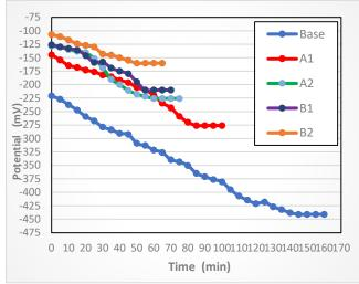
Figure 6. OCP-time of TiO<sub>2</sub>, and ZrO<sub>2</sub>/TiO<sub>2</sub> coating by PEO process in Hank's solution.
