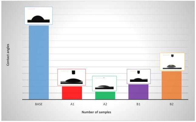
Figure 5. Results of contact angle of base, TiO<sub>2</sub>, and ZrO<sub>2</sub>/TiO<sub>2</sub> coating by MAO process at 400V with different times in Hanks's solution.
