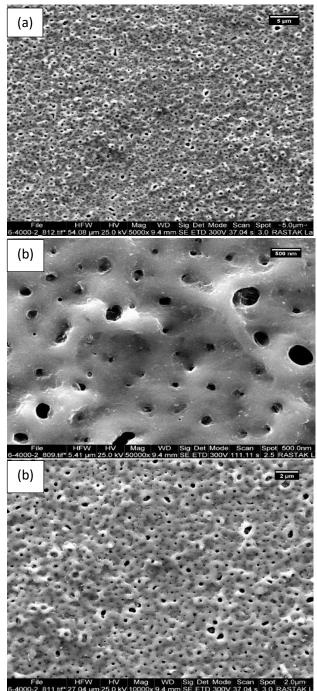
Figure 2. FESEM micrographs of  $TiO_2$  coating by PEO process (a) at 5min, and (b) 10min.
