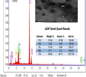
Figure 4. EDS result of TiO<sub>2</sub>, and ZrO<sub>2</sub>/TiO<sub>2</sub> by PEO Process with different time (a) A1 sample, (b) A2 sample, (c) B1 sample, and (d) B2 sample.
