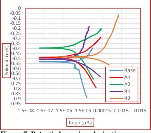
Figure 7. Potentiodynamic polarization curves of TiO<sub>2</sub>, ZrO<sub>2</sub>/TiO<sub>2</sub> coated by PEO process and base at different time and applied voltages 400V in Hank's solution.
