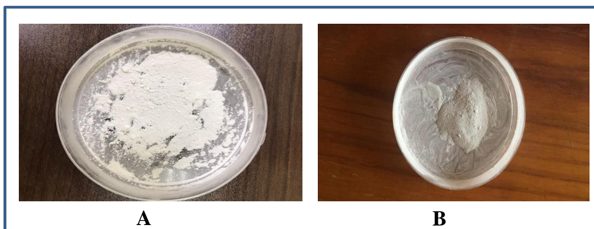
Figure 2. The final white powder of TiO 2 prepared by A) sol-gel method and B) green method.
