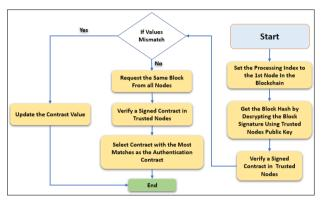
Figure 10. Flowchart of blockchain verification in trusted node.
