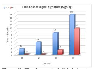
Figure 19. The time cost of digital signature (signing).
