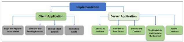
Figure 2. The implementation of client and server applications.
