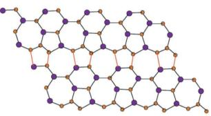
(a) One row of  $Si_2C_3$ -I[t, h] (b) Connection of two rows of  $Si_2C_3$ -I[t, h] Figure 2. 2D structure of  $Si_2C_3$ -I[t, h]. (a)  $Si_2C_3$ -I[t, h], one row with t = 4 and h = 1; (b)  $Si_2C_3$ -I[4, 2], two rows are being joined together. The upper and lower rows are interlinked by red lines (edges).
