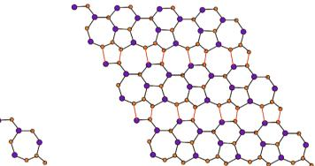
(a) Unit cell of Si<sub>2</sub>C<sub>3</sub>-I[t, h] (b) Si<sub>2</sub>C<sub>3</sub>-I[4, 3]. Figure 1. 2D structure of Si<sub>2</sub>C<sub>3</sub>-I[t, h]. (a) A chemical unit cell of Si<sub>2</sub>C<sub>3</sub>-I[t, h]. Si<sub>2</sub>C<sub>3</sub>-I[4, 3]. The carbon atom C is brown, while the silicon atom Si is blue
