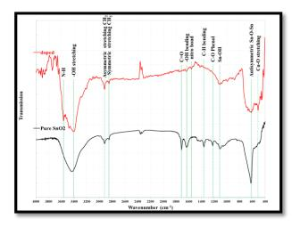
Figure 6. FTIR spectra of pure tin oxide nanoparticles synthesized by active biosynthesis using eggshell membrane
