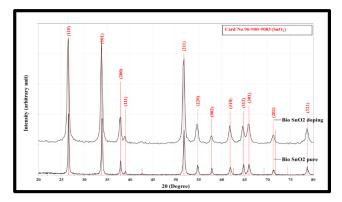
Figure 1. X-ray diffraction pattern of a) pure Sno<sub>2</sub> nanoparticles .b) SnO2 NPS doped with Cu 2%
