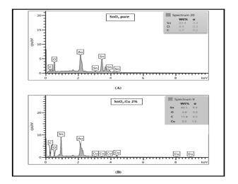
Figure 4. EDX image of. A) Pure SnO<sub>2</sub>. B) SnO<sub>2</sub>: 2% Cu
