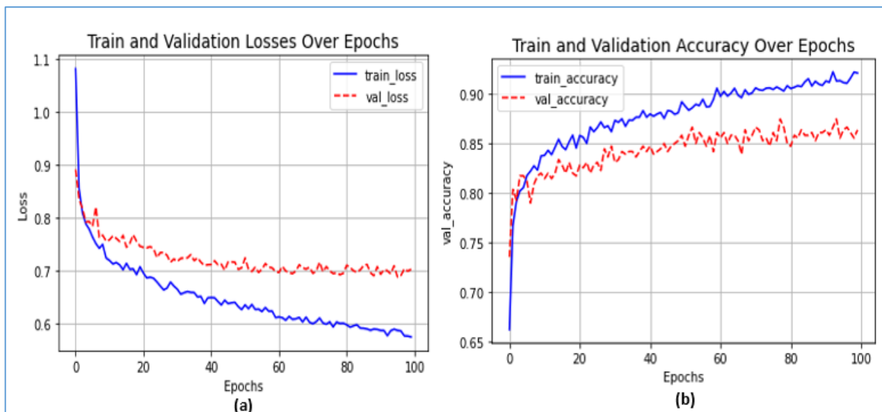
Figure 10. Training and validation over epochs for APTOS 2019 dataset, (a)loss, (b) accuracy, (epochs=100), WT Attention-Db5 Block-Swin-B to multi-class.
