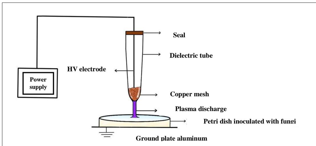
**Figure 1. Schematic representation of the experimental set-up of the dielectric barrier discharges (DBD) plasma reactor for plasma treatment of fungi. A high-voltage electrode is connected to a copper mesh to scatter the discharge over the entire area of the dielectric barrier. The sample is placed on an aluminum stage and the discharge occurs between the bottom surface of the quartz tube and the top surface of the sample, which are separated by a distance of 5 mm.**
