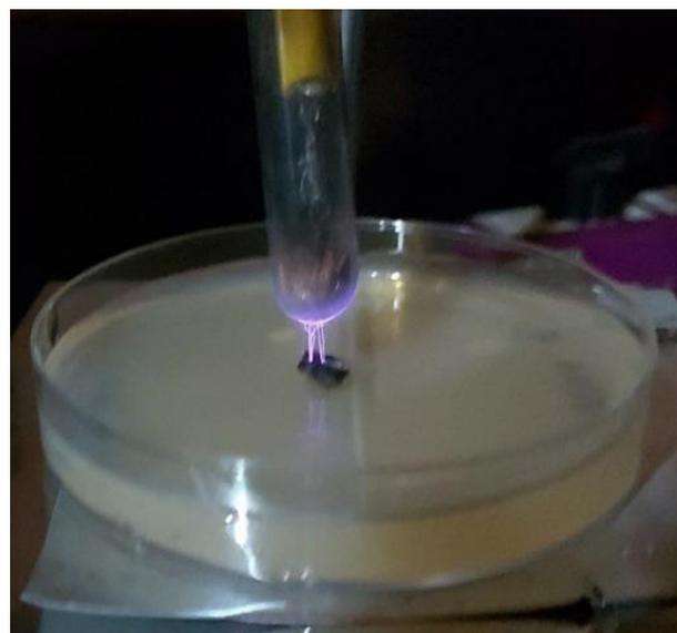
**Figure 2. Photograph of a fungal sample in a petri dish during exposure to DBD plasma treatment. Statistical analysis**
