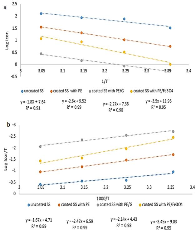
**Figure 4. A graph showing: a. log Icor. Against 1/T for SS316L with coating by PE/G, Fe<sub>3</sub>O<sub>4</sub>, b. log I<sub>cor.</sub>/T versus 1000/T SS316L for with coating by PE/G, Fe<sub>3</sub>O<sub>4</sub>.**
