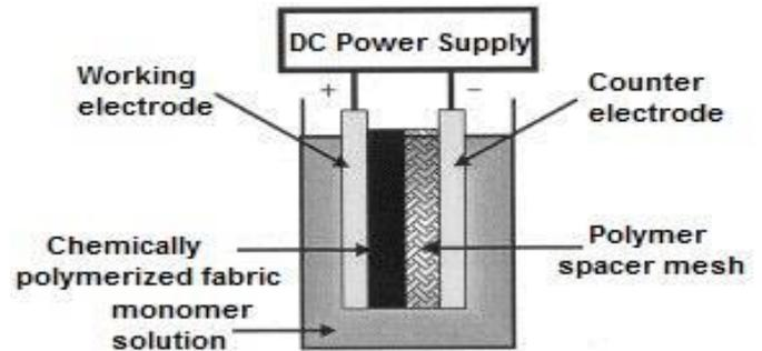
Figure 1. Electropolymerization system
