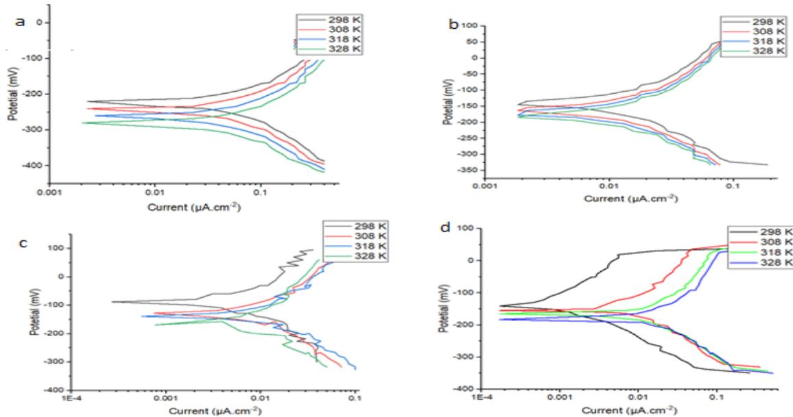
**Figure 2.** Shows the Tafel curves for corrosion of the following materials: a. untreated alloy, b. coating PE, c. coating PE/ G, and d. coating PE/Fe<sub>3</sub>O<sub>4</sub>.
