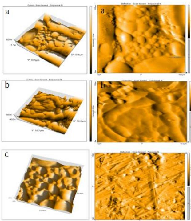
**Figure 5. AFM Images of, a. PE, b. PE/G, c. PE/Fe<sub>3</sub>O<sub>4</sub>.**
