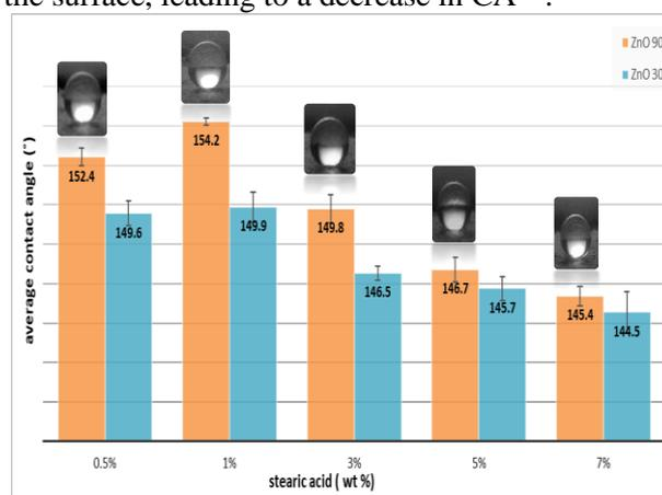
Figure 4. Effect of stearic acid on contact angle
