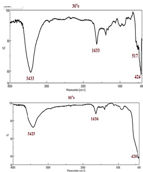
**Figure 2.** FTIR spectrum of the synthesis ZnO NPs
