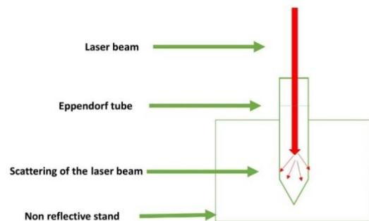
**Figure 2. Arrangement of laser irradiation**
