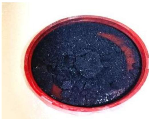
**Figure 2. Shows the raw materials after washing by hexane solvent**
