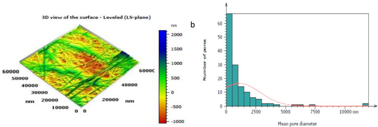
**11b. AFM image and porosity histogram of PVA + PA+0.01 wt% nanofibers**
