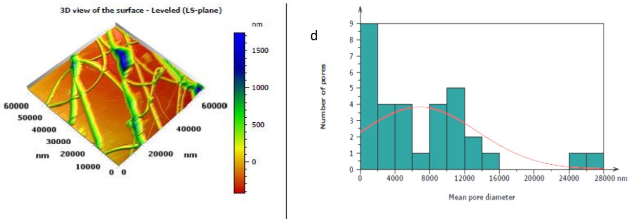
**11.d AFM image and porosity histogram of PVA + PA+0.03 wt% nanofibers**
