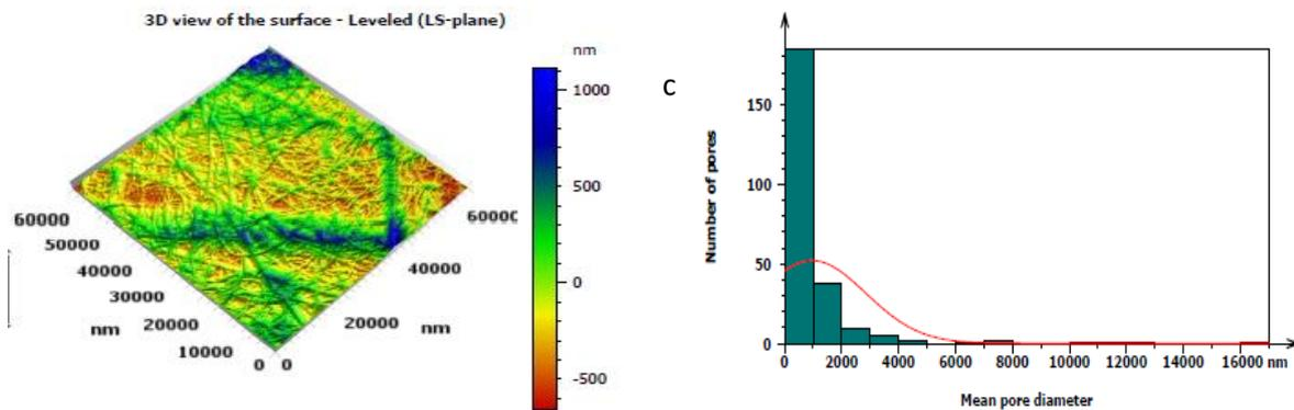
**11.c AFM image and porosity histogram of PVA + PA+0.02 wt% nanofiber**
