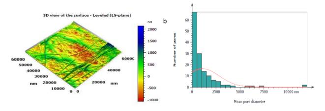
11b. AFM image and porosity histogram of PVA + PA+0.01 wt% nanofibers
