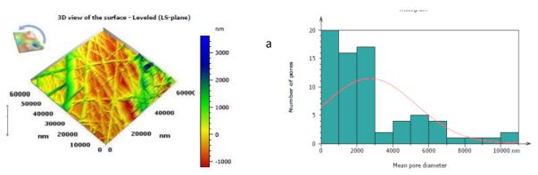
11a .AFM image and porosity histogram of Pure PVA + PA nanofibers
