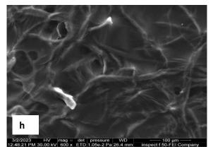
SEM of PA+PVA + 0.3 wt% CNP filter before flirtation Figure 10. (a-h). SEM images of Nanofibers samples SEM of PA+PVA + 0.3 wt% CNP filter after flirtation
