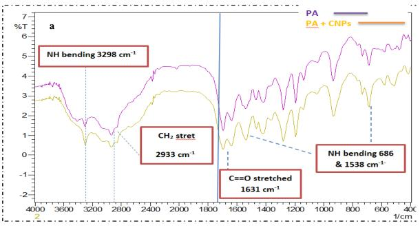
Figure 7 a. FTIR analysis of PA and PA+CNPs
