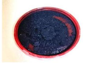
Figure 2. Shows the raw materials after washing by hexane solvent
