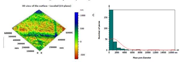
11.c AFM image and porosity histogram of PVA + PA+0.02 wt% nanofiber
