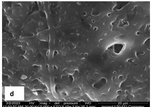
SEM of PA+PVA+0.1 wt% CNP filter after flirtation
