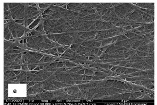
SEM of PA+PVA + 0.2 wt% CNP filter before filtration
