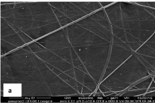
SEM of PA+PVA filter before fliration
