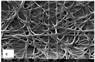
SEM of PA+PVA+0.1wt% CNP filter before flirtation
