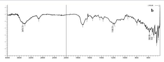
Figure 7b. FTIR analysis of PVA+PA blend nanofibers (matched with Darwish et al.<sup>21</sup>)
