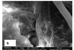
SEM of PA+PVA filter after fliration
