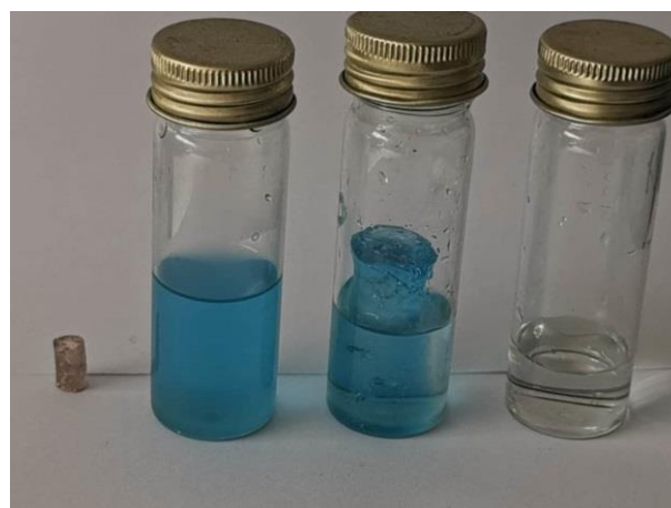
Figure 11. Photograph of right to left: Synthesized poly TBA/OA, \text{Cu}^{+2} solution, swollen polymer adsorbs \text{Cu}^{+2} , and purified water
