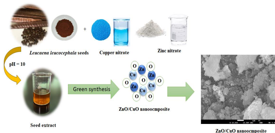
Scheme 1. Schematic steps for the green synthesis of ZnO/CuO nanocomposites
