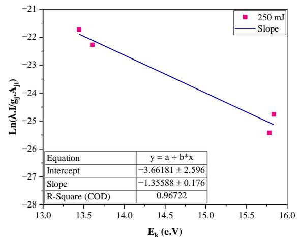
Figure 4. Boltzmann plot for 4 neutral and ion c spectral lines at laser energy range 250-500 mJ using  $\lambda$  532 nm
