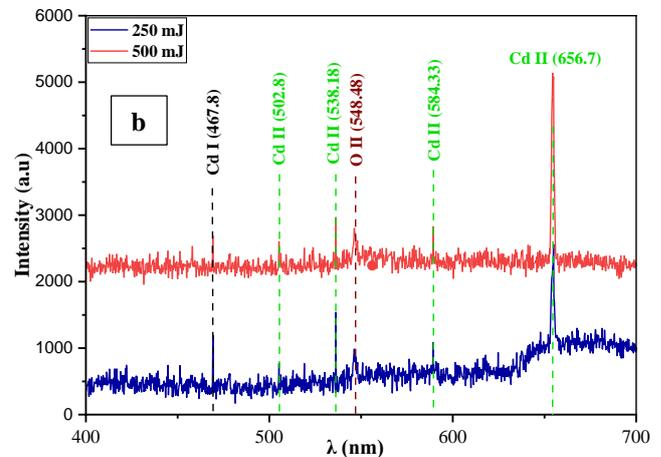
**Figure 2.** Displays the emission spectra of Cadmium plasma inside a distinct window, encompassing the spectral ranges of 400 to 700 nm. These spectra are generated by the utilization of the (a) first harmonic 1064 nm and (b) second harmonic 532 nm of the laser for different laser energy.
