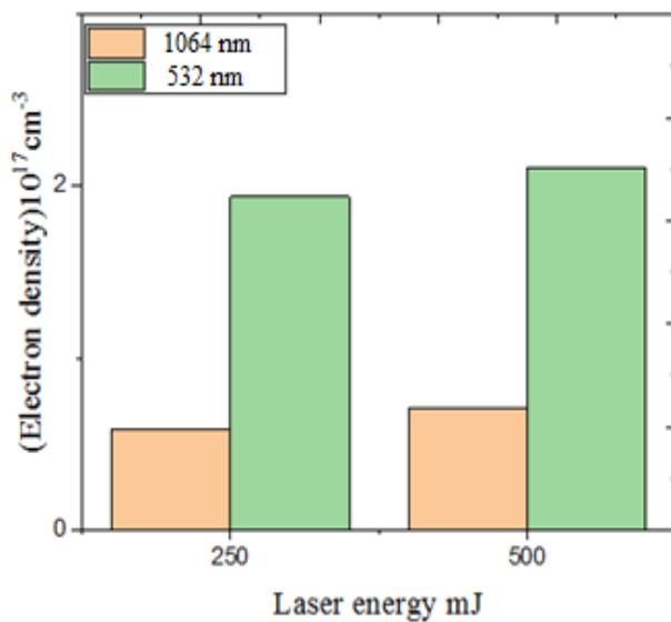
**Figure 7. The electron density at  $\lambda$  1064 and 532 nm as a function of laser energy**
