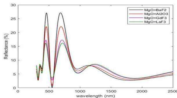
**Figure 4. Irregular behaviours of the reflection peak in the visible region for the four coatings using the second optical design (Glass/L/H/L/H/L).**
