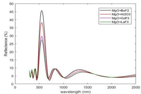
**Figure 3. Behaviour of the reflection peak in the visible region for four coatings using the first optical design (Glass/H/L/H/L/H).**
