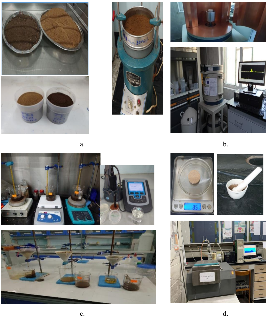
Figure 2. a. samples preparation b. gamma-ray spectroscopy c. the chemical washing and pH meter d. XRF-system and sample preparation
