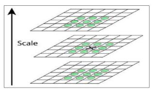
Figure 6. "Pixel assessments to find the difference-of-Gaussian image's maximum and minimum values"
