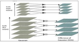
Figure 5. Construction of difference-of-Gaussian images
