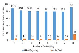
Figure 11. The backwashing cycles of 11 wt.% PAN/DMF membrane (Feed flowrate= 60 ml/min, feed oil concentration = 250 mg/L, transmembrane pressure = 1.5 psi, and temperature=  $25^{\circ}$ C)
