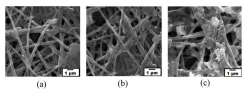
Figure 10. The SEM images of the 11% PAN/DM EPNF membranes (magnification is 10000 X) after emulsified oil removal under various transmembrane pressures (a) 1.5 psi, (b) 5 psi, and (c) 10 psi.
