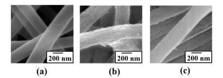
Figure 12. High resolution SEM images of the surface of 11 wt. % PAN/DMF membrane (magnification is 160000 X) (a) Clean membrane (b) Fouled membrane, and (c) Backwashed membrane
