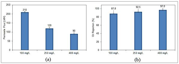
Figure 7. The separation efficiency of 11% PAN/DMF EPNF membrane under various feed oil concentrations (Feed flowrate= 60 ml/min, transmembrane pressure = 1.5 psi, and temperature=  $25^{\circ}$ C) (a) Permeate flux and (b) Oil rejection
