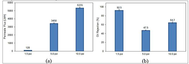
Figure 9. The separation efficiency of 11% PAN/DMF membrane under various transmembrane pressures (Feed flowrate= 60 ml/min, feed oil concentration = 250 mg/L, and temperature= 25°C) (a) Permeate flux and (b) Oil rejection
