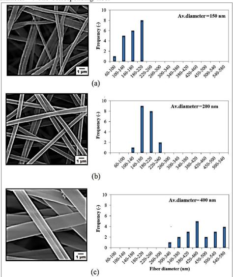
Figure 2. SEM images of PAN-based EPNF membranes (magnification is 10000 X) and the corresponded fiber size prepared from different PAN/DMF concentrations (a) 8%PAN/DMF, (b) 11%PAN/DMF, and (c) 14%PAN/DMF.
