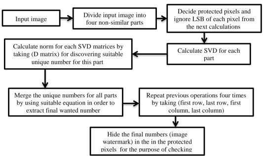
Figure 7. Block diagram of the proposed system
