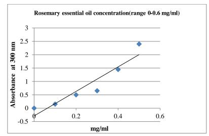
Figure 2. Calibration curve for evaluation rosemary essential oil concentration.
