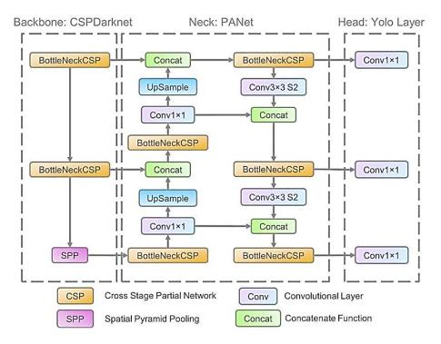
Figure 3. The network architecture of YOLOv5<sup>18</sup>.
