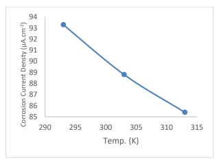
Figure 2. Effect of temperature on the corrosion current density of carbon medium in (1) M of HCl acid
