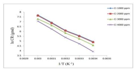
Figure 24. Diagram showing the corrosion of medium carbon steel at different concentrations of kujurat extract at different Temp.
