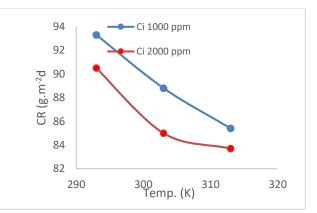
Figure 4. The effect of temperature effect on the corrosion rate of medium carbon steels in (1) M HCl with the presence of aqueous
