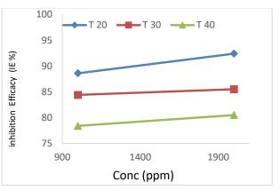
Figure 10. Effect of concentration on inhibition efficiency in (1) M HCl
