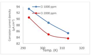
Figure 5. Effect of temperature on the density of the corrosion current in 1M HCl with an aqueous extract
