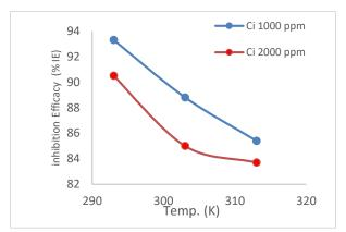
Figure 8. Effect of Temperature on the inhibition efficiency (1) M HCl in presence of alcoholic extract
