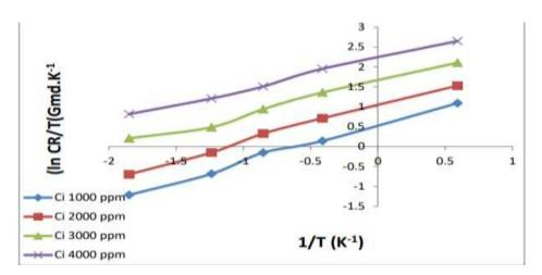
Figure 23. Transitional state of corrosion of medium carbon steel in the presence and absence of Kujarat Tea Plant
