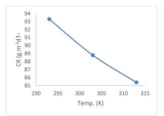
Figure 1. Effect of temperature on the Corrosion Rate carbon steel in (1) M of HCl acid
