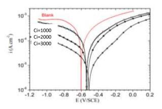
Figure 22. Polarization curves of medium carbon steel the presence of different concentrations of Kujarat Tea Plant
