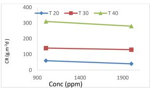
Figure 14. Effect of Concentration on Corrosion rate in (1) M HCl with alcoholic extract.
