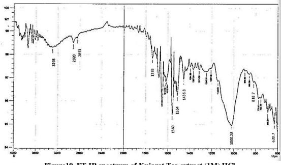
Figure19. FT-IR spectrum of Kujarat Tea extract (1M) HCl
