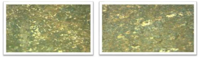
1000ppm 2000ppm Figure 18. SEM electron Microscopy images of steel after corrosion in 1M HCl in the presence of alcoholic extract (1000ppm) extract in concentration (1000, 2000ppm)
