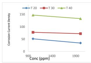
Figure 12. Effect of concentration on density of the erosion current in (1) M HCl with the presence of the alcoholic extract
