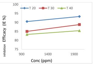
Figure 9. Effect of concentration on inhibition efficiency in (1) M HCl
