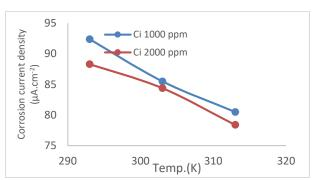
Figure 6. Effect of temperature on density of the corrosion current in (1) M HCl in presence of the alcoholic extract
