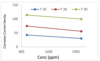
Figure 11. Effect of concentration on density of the erosion current in (1) M H with a aqueous extract
