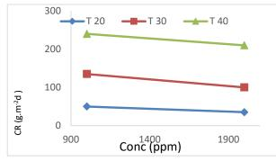
Figure 13. Effect of Concentration on The corrosion rate in (1) M HCl with aqueous extract
