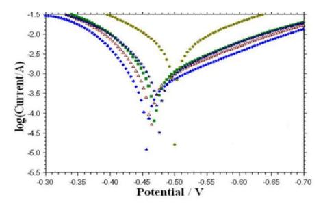
Figure 21. Tifel curves: Increasing Kujarat Tea Plant concentrations (1000,2000,3000) ppm on the corrosion of medium carbon steel in solution 1M HCl
