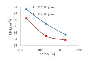
Figure 3. The effect of Temperature rate of medium Carbon in (1) M HCl with the presence of on extract alcoholic extract
