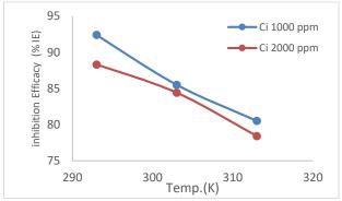
Figure 7. Effect of Temperature on inhibition efficiency in (1) M HCl in presence of aqueous extract
