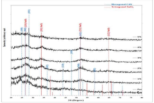
Figure 1. XRD spectrum of the CdS pure and doped with concentrations 1, 2, 3, 4, and f:5 wt. % Sn nanoparticles.
