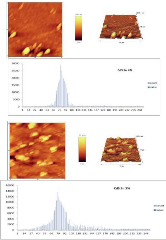
Figure 3. AFM images describing the surface morphology for CdS the pure and CdS nanoparticles doped with 1, 2, 3, 4, and 5 wt. % Sn.
