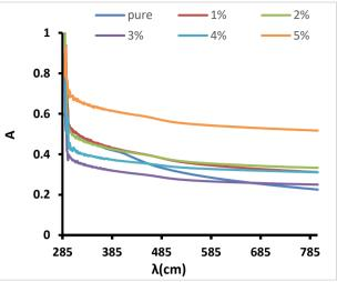
Figure 4. Uv-Vis spectrum of pure CdS and doped d with (1, 2, 3, 4, and 5) % wt. Sn nanoparticles.
