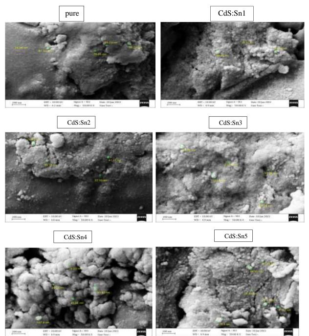
Figure 2. SEM images for CdS NPs pure and doped with 1,2,3,4,5 wt% Sn
