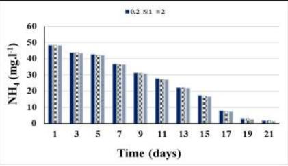
Figure 4. Effect of adding different doses of micro-algae *Coelastrella* sp. (0.2, 1, and 2 g. l<sup>-1</sup>) on ammonium content values of wastewater.
