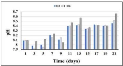
Figure 1. Effect of adding different doses of micro-algae *Coelastrella* sp. (0.2, 1, and 2 g. l<sup>-1</sup>) on pH values of wastewater.
