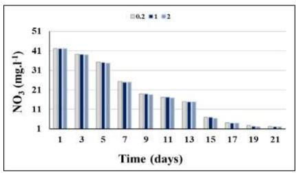
Figure 5. Effect of adding different doses of micro-algae *Coelastrella* sp. (0.2, 1, and 2 g. l<sup>-1</sup>) on nitrate content values of wastewater.
