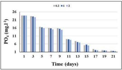
Figure 6. Effect of adding different doses of micro-algae *Coelastrella* sp. (0.2, 1, and 2 g. l<sup>-1</sup>) on phosphate content values of wastewater.
