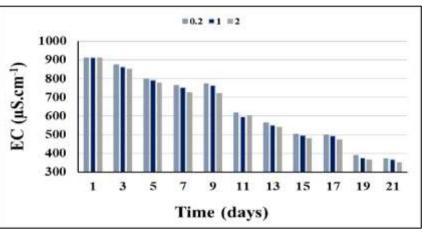
Figure 2. Effect of adding different doses of micro-algae *Coelastrella* sp. (0.2, 1, and 2 g. l<sup>-1</sup>) on electrical conductivity values of wastewater.
