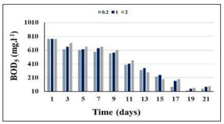
Figure 3. Effect of adding different doses of micro-algae *Coelastrella* sp. (0.2, 1, and 2 g. l<sup>-1</sup>) on BOD<sub>5</sub> values of wastewater.
